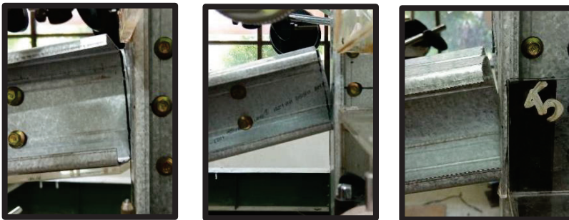
Fig. 2. Failure at the screw joint.
