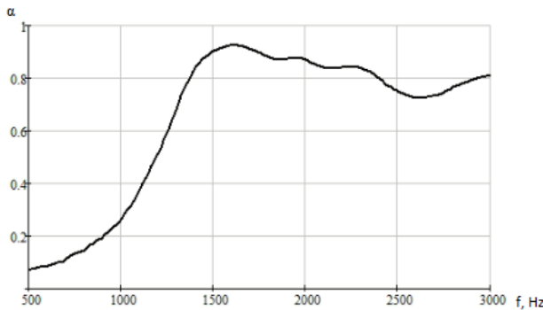
Fig. 3. The graph of the dependence of the acoustic efficiency on the natural frequency of the different-height SAS.
