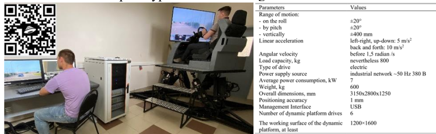
Fig. 5. a) a prototype of an automotive driving simulator with an integrated system of virtual 3D models of real terrain; b) technical characteristics of the automotive driving simulator.
