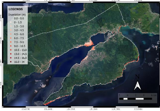
Fig. 3. Tsunami inundation based on the numerical simulation with magnitude 9,1 Mw
