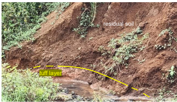
Fig. 8. Light brown tuff layer exposed at the toe side of Rawacina Landslide underneath the completely weathered breccia's light to dark residual soil.
