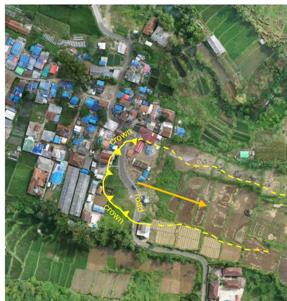
Fig. 6. UAV image of Sarampad landslide showing the gentle slope morphology of the head scarp area.
