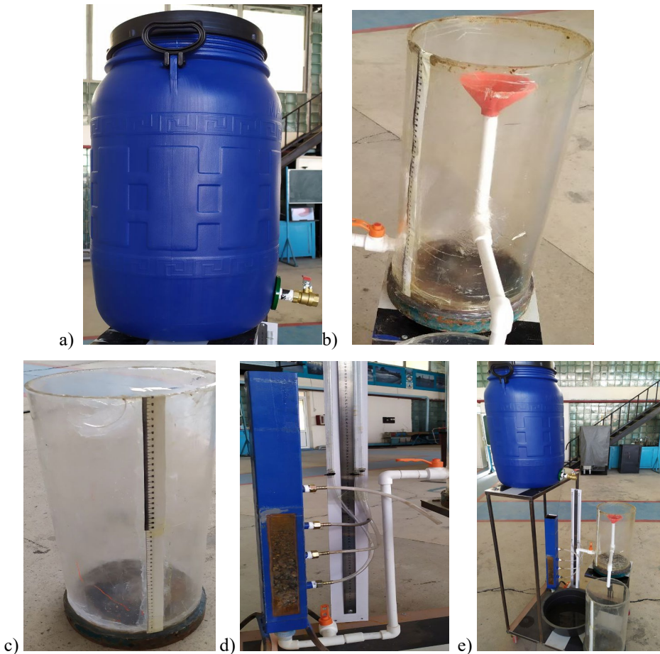
Fig. 2. Model of laboratory local treatment facilities with vertical settling tanks: a) wastewater tank; b) vertical sump; c) flakes and oil storages; d) filter e) model of local treatment facilities with vertical settling tanks.
