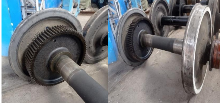
Fig. 1. A toothed wheel of integral construction in the wheel-motor unit of main locomotives
