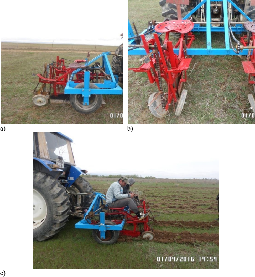
Fig.4. A layout sample of a two-row combined tool. a –side view; b – rear view; c – the technological process of the tool.
