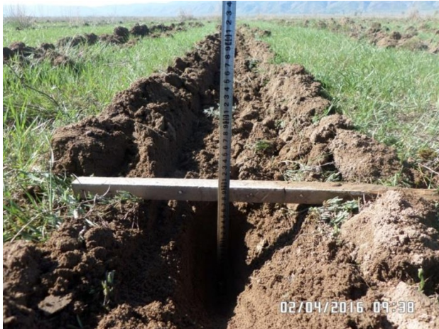
Fig. 5. Measuring the depth of tillage
