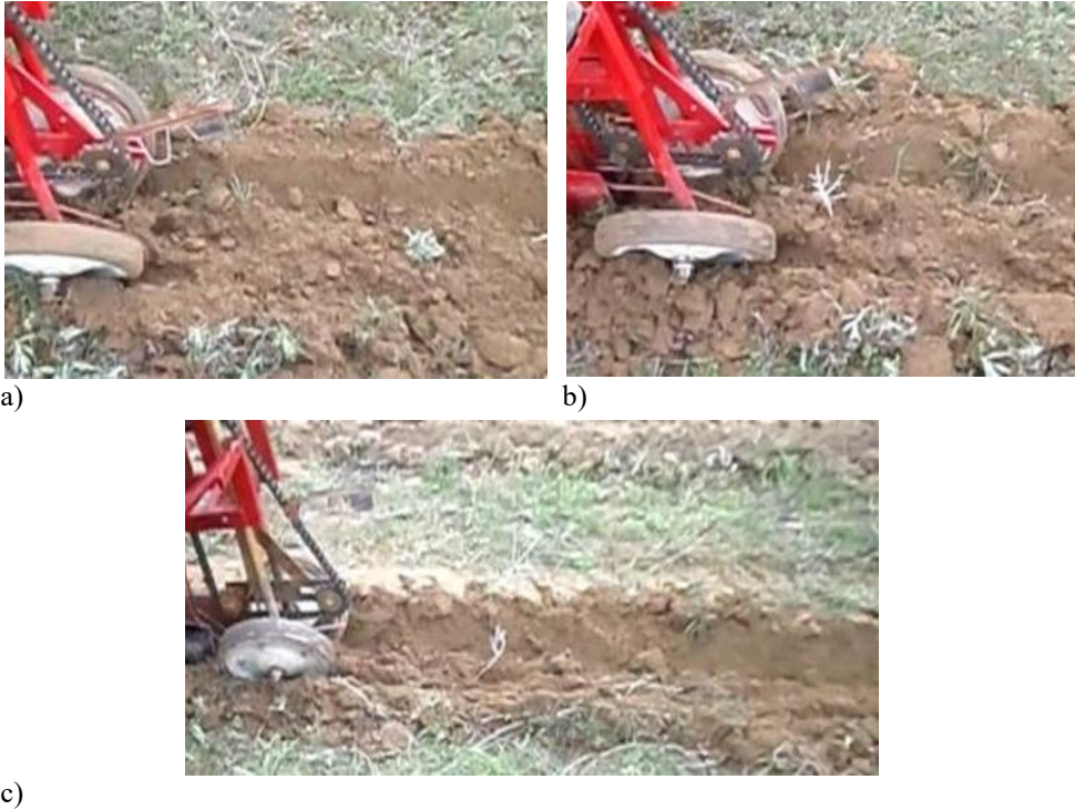
Fig. 6. General view of planting process, a) at a speed of 0.84 m / s. b) at a speed of 1.12 m / s. c) at a speed of 1.4 m / s
