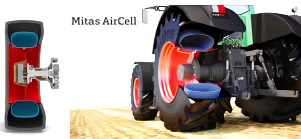
Fig. 9. Mitas Aircell tyre principle of operation.
