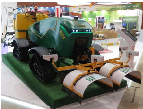
Fig. 1. Multifunctional robotic device with an intelligent vision system
